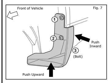
Push splash guard upward and inward towards vehicle and tighten the two (2) screws and one (1) bolt in the sequence shown.
