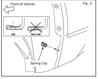
4) Install one (1) Spring Clip over 6mm drilled hole as shown.
